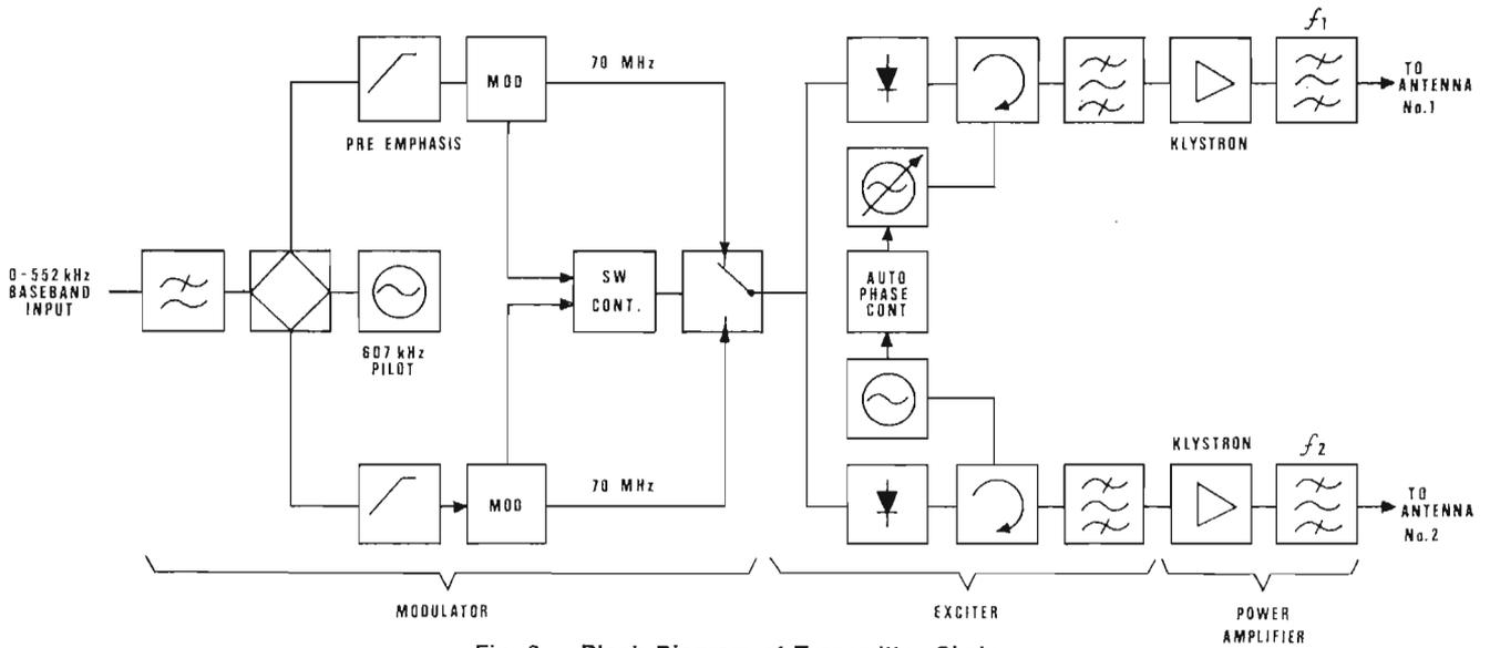
Fig. 8 — Block Diagram of Transmitter Chain.
