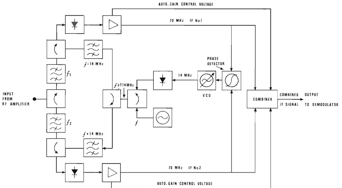
Fig. 9 — Block Diagram of Receiver.
