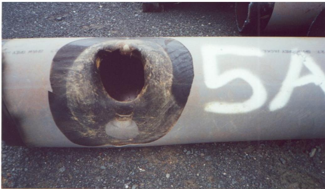
**Figure 3: Puncture from D6H Bulldozer Ripper**
