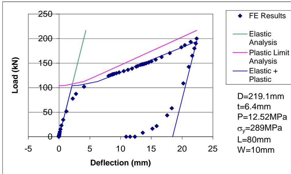
This chart shows the deformation commencing at the left hand side and the change in the load for the various types of deformation up to the point of puncture when the deformation load reduces as shown on the right hand side of the chart.
