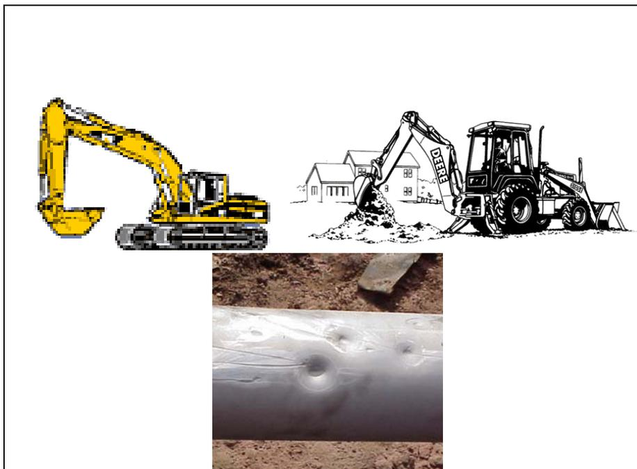
**Figure 1: Excavator Damage**
